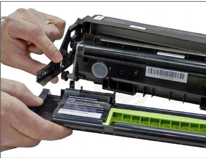
2. Pull the edge of the frame out slightly and remove the handle.
