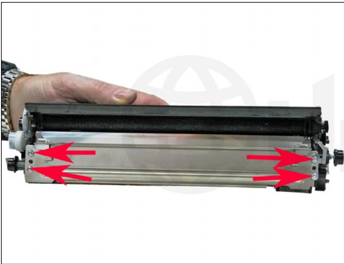
20. Using a size T-10 Torx screwdriver, remove the four screws from the doctor blade.
