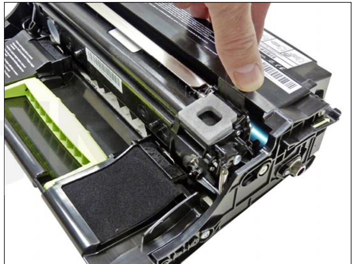
The toner cartridges feed the toner to the drum units through a small toner port.
