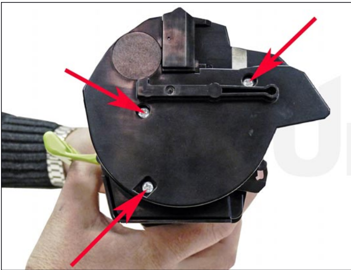
10. Install the end cap and three screws.
